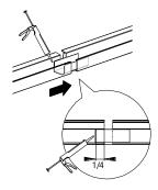
**4.** Insert the second gutter ¼ of the way into the other side of the connector and sealant the edge.
