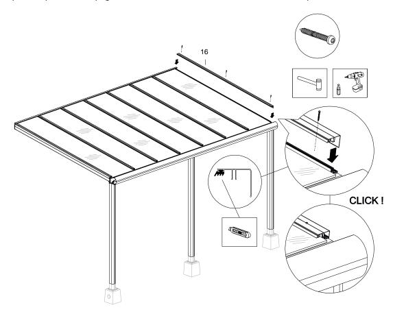
**10.** Now screw a sheet stopper at the gutter end of each middle beam to ensure secure attachment. **Note:** securing the end cover strips comes later.
