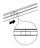
**5.** Now press the second gutter completely over the gutter extension to form a seamless joint between the gutters.
