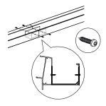
**6.** The gutter extension can now be secured with the short stainless steel screws in the chamber of the gutter and on the front side under the decorative profile. Apply sealant on the assembly so it is smooth and waterproof!
